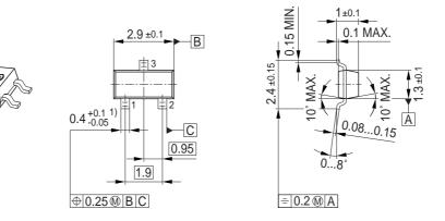
1) Lead width can be 0.6 max. in dambar area
